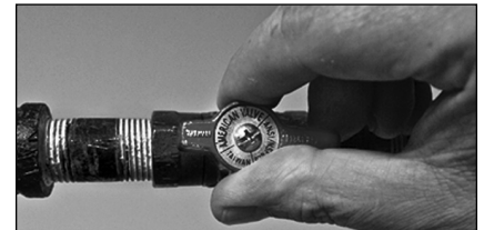
Figure 58 - Gas valve in “on” position.
